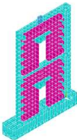
Fig. 26.C. Typical meshing (Doors opening).
