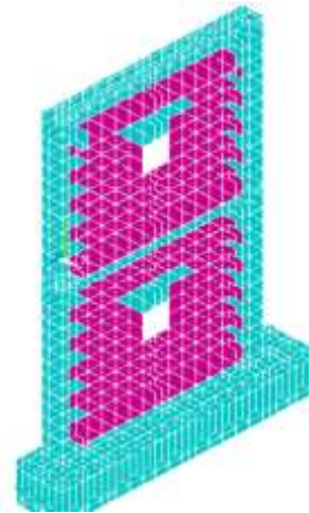
Fig 26.D. Typical meshing (Windows Opening)
