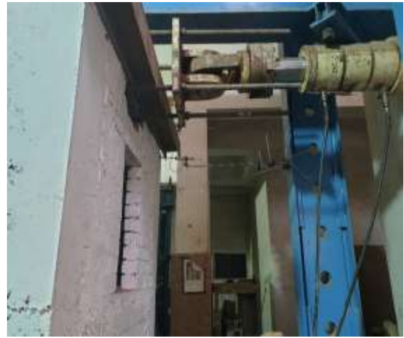
Fig 5. Hydraulic jack fixed at roof level.
