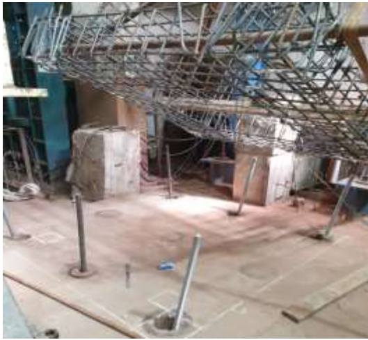
Fig. 4. Fixing the raft to the reaction floor.
