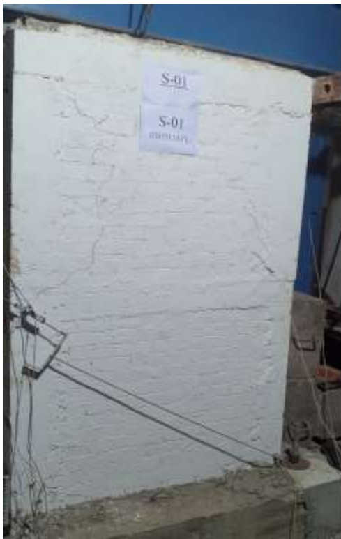
Fig.11. DS1 first cracks at upper floor
